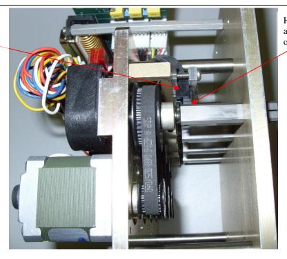
Home position marker – at least half way into the optical sensor!
