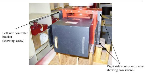
Remove right and left side controller brackets unfastening 2 Phillips screws per bracket as shown in the picture above.
