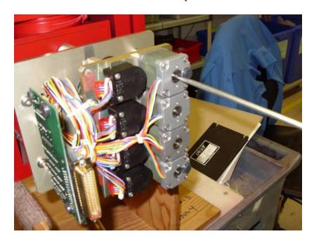
If the motors are struggling to execute this command, give them a helping hand. A gentle turn of the struggling pulley in the same direction the motor is trying to turn should suffice. Be extremely careful doing this!
