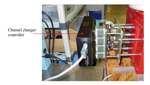
Plug the klystron's channel changer controller (make sure D50 connector is fully engaged) back into the motor module assembly as shown in the picture above. Use PC interface cable supplied with each klystron (CPI P/N 764058). Plug the DB15 (f) connector marked "CONTROLLER" into the DB15 (m) port on the channel changer controller assembly. Connect DB15 (m) connector marked "A2J7" to the cable coming
