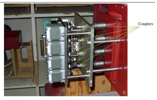
The picture above shows tuner (motor module) with cover removed (couplers in the highest frequency position).
