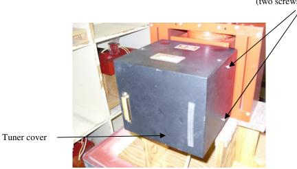
Tuner cover right side screws (two screws also on left side)
